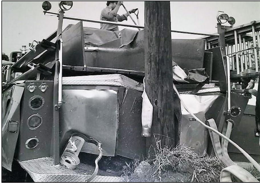
Fire truck spun 360 degrees before striking utility pole after impact with automobile.
